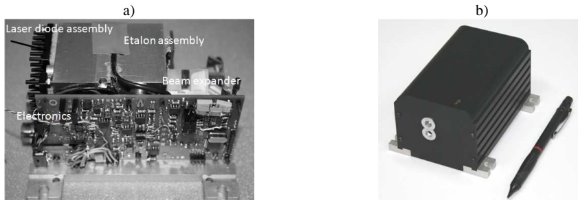
Fig. 1. LD interferometer head. a) internal b) general view of the head.
